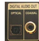
Example of Digital Audio Output socket on TV. The Optical output is normally protected by a hinged cover plate.
